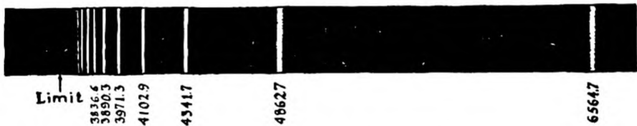
FIG. 8-6 The Balmer series of spectral lines of atomic hydrogen. The line at the right, with the longest wavelength, is H\alpha . It corresponds to the transition from the state with n = 3 to the state with n = 2 .
